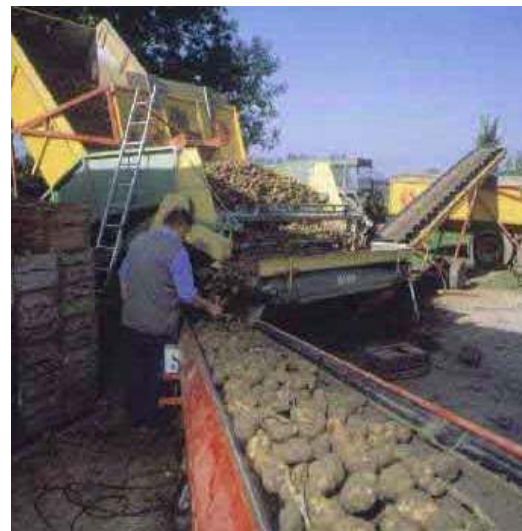
Potatoes are often unloaded into a hopper from which they are transferred to a pre-cleaner which removes still more earth and small tubers.
